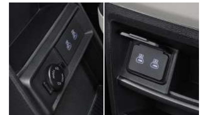
USB Type-C Ports (Front: 1 Charging, 1 Data & Charging / Rear: 2 Charging)
